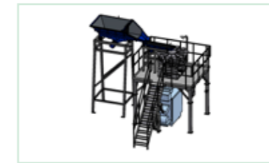
With success both a linear and a Multihead Weigher have been installed.
