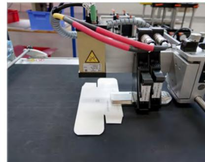
Print process of the non erected carton
